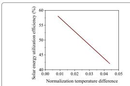
**Fig. 4** Relationship between normalization temperature and solar energy utilization efficiency
