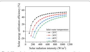
**Fig. 9** Effect of solar radiation intensity on solar energy utilization efficiency
