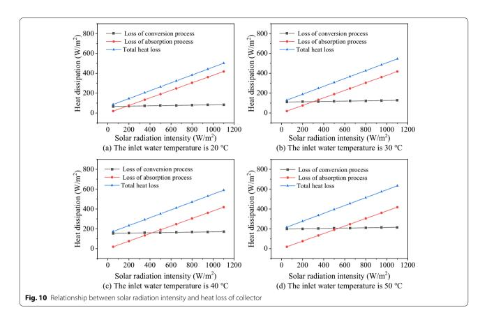
can improve the thermal performance of the collector. If solar irradiation is weak, it can be considered to improve the absorptivity of the collector and reduce the heat loss to promote SEUE. When solar irradiation is strong, the effect of improving the absorptivity of the collector is more significant.
