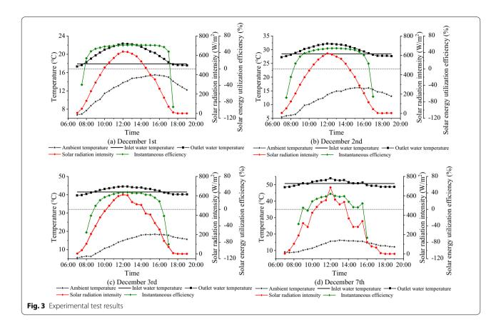
gradually decreases from 13.7 °C to 10.0 °C from 17:50 to 20:50, and the outlet water temperature of the collector decreases from 17.7 °C to 17.5 °C.
