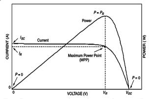
**Fig. 1** Characteristic power–voltage and current–voltage curves (Tse et al. 2002)
