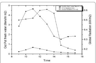
**Fig. 4** Hourly variation of distil water w.r.t global radiation and wind speed
