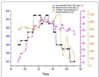
**Fig. 3** Hourly variation of experimental various temperature of solar distillation system in 22nd March
