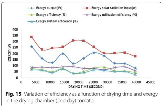
**Fig. 15** Variation of efficiency as a function of drying time and exergy in the drying chamber (2nd day) tomato
