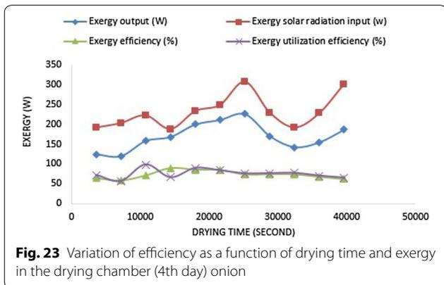
221.5 and 310.3 W on the first day, 179.2 W to 301.8 W on the second day and 171.1 W to 1084.6 W On the third day and 188.2 W to 307.7 W on the fourth day depending on the experimental condition of potato. Figures 20, 21, 22 and 23 show the exergy utilization efficiency calculated by using Eq. (16). It was dependent on the exergy solar radiation input and exergy output. The exergy
