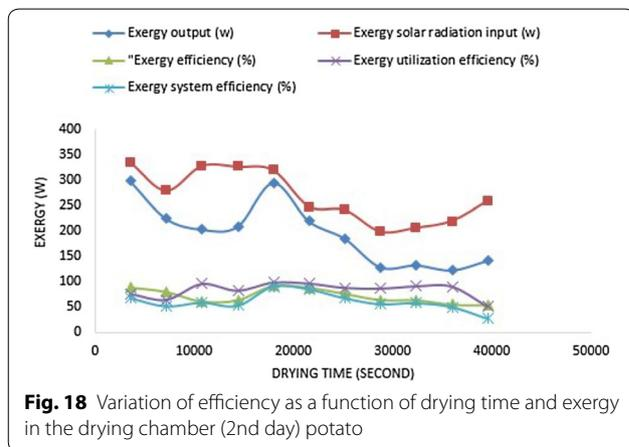
**Fig. 18** Variation of efficiency as a function of drying time and exergy in the drying chamber (2nd day) potato
