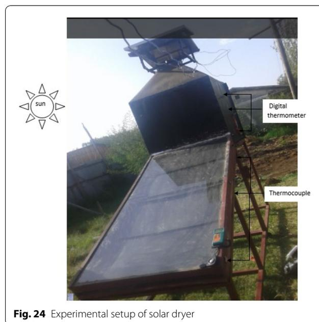
**Fig. 24** Experimental setup of solar dryer
