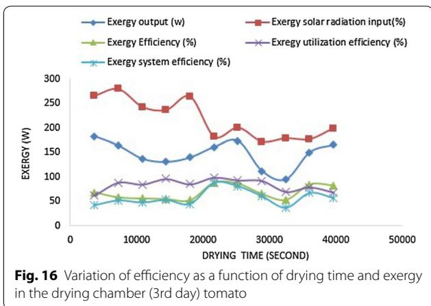
**Fig. 16** Variation of efficiency as a function of drying time and exergy in the drying chamber (3rd day) tomato
