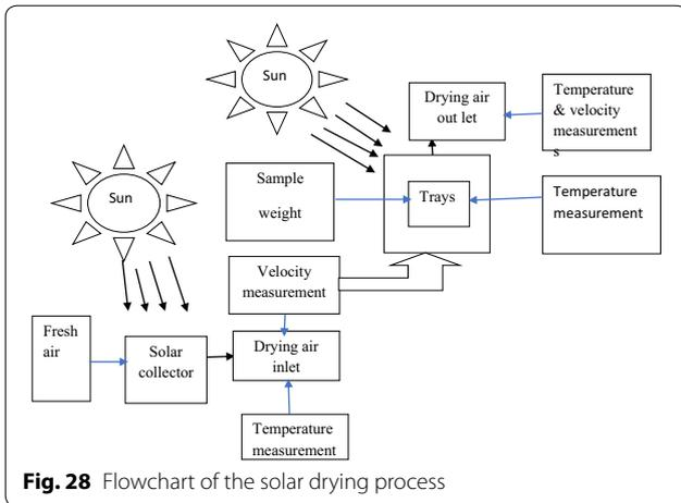
**Fig. 28** Flowchart of the solar drying process
