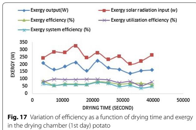
**Fig. 17** Variation of efficiency as a function of drying time and exergy in the drying chamber (1st day) potato
